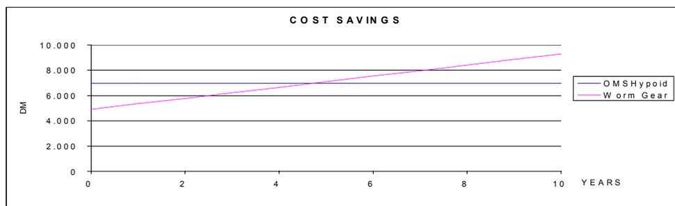
Remark: The Difference in the investment of the *OMSHypodrive* and Worm Gear Drive is approximaletly 30%. The additional energy costs of the worm gear drive compared to the *OMSHypodrive* (app. DM 440,- / year) are determining the ascending of the worm gear graph. Example given is for escalator for commercial applications.
