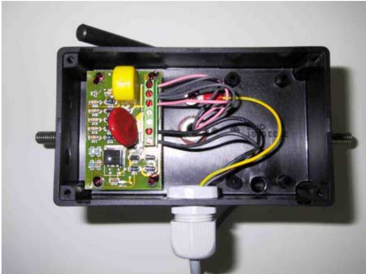
Picture: O20 Braking Solenoid, view into the opened junction box shows the electronic control module. All braking solenoids are available with CSA approval.
