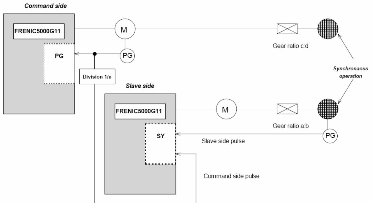
Figure 4. Example system setup.
