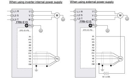
Figure 2.3 Connection Diagrams for Compliance with EMC Directive
