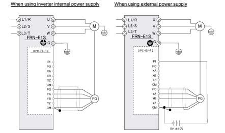
Figure 2.2 Connection Diagrams for Speed Control with PG and Positioning Control
