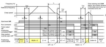
Figure 7.2 Positioning Control Status Transition Model
