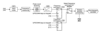
Figure 5.4 Block Diagram of the Pulse Train Input System
