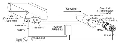
Figure 6.1 Speed Control Model Using a PG
