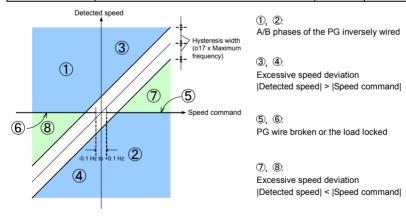
Figure 8.1 Excessive Speed Deviation Detection and Speed Command
