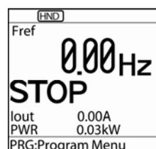
Figure 4.2 Display of the LCD Monitor after Power-ON
