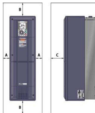
Figure 2.1 Mounting Direction and Required Clearances
